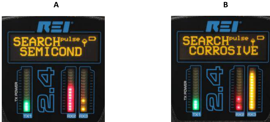
ORION 2.4 COMPARISON OF HARMONIC LEVELS (A – Semiconductor, B – False Junction; Bargraphs on the right are the 2 nd and 3 rd harmonic levels)
